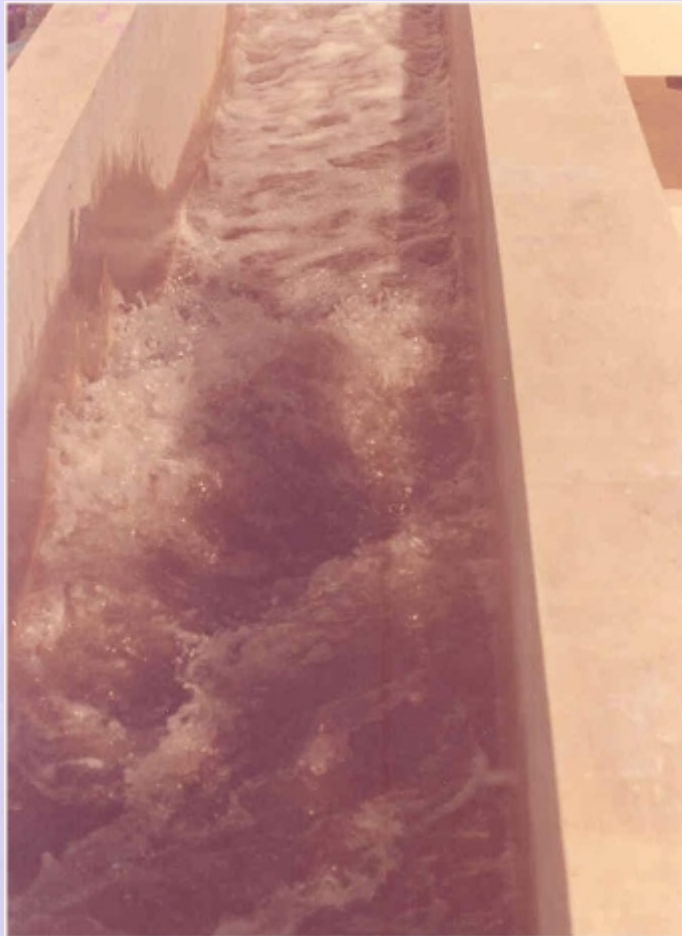
Concrete Flume - Super Critical Flow (2 m 3 /s, 1 m width)
